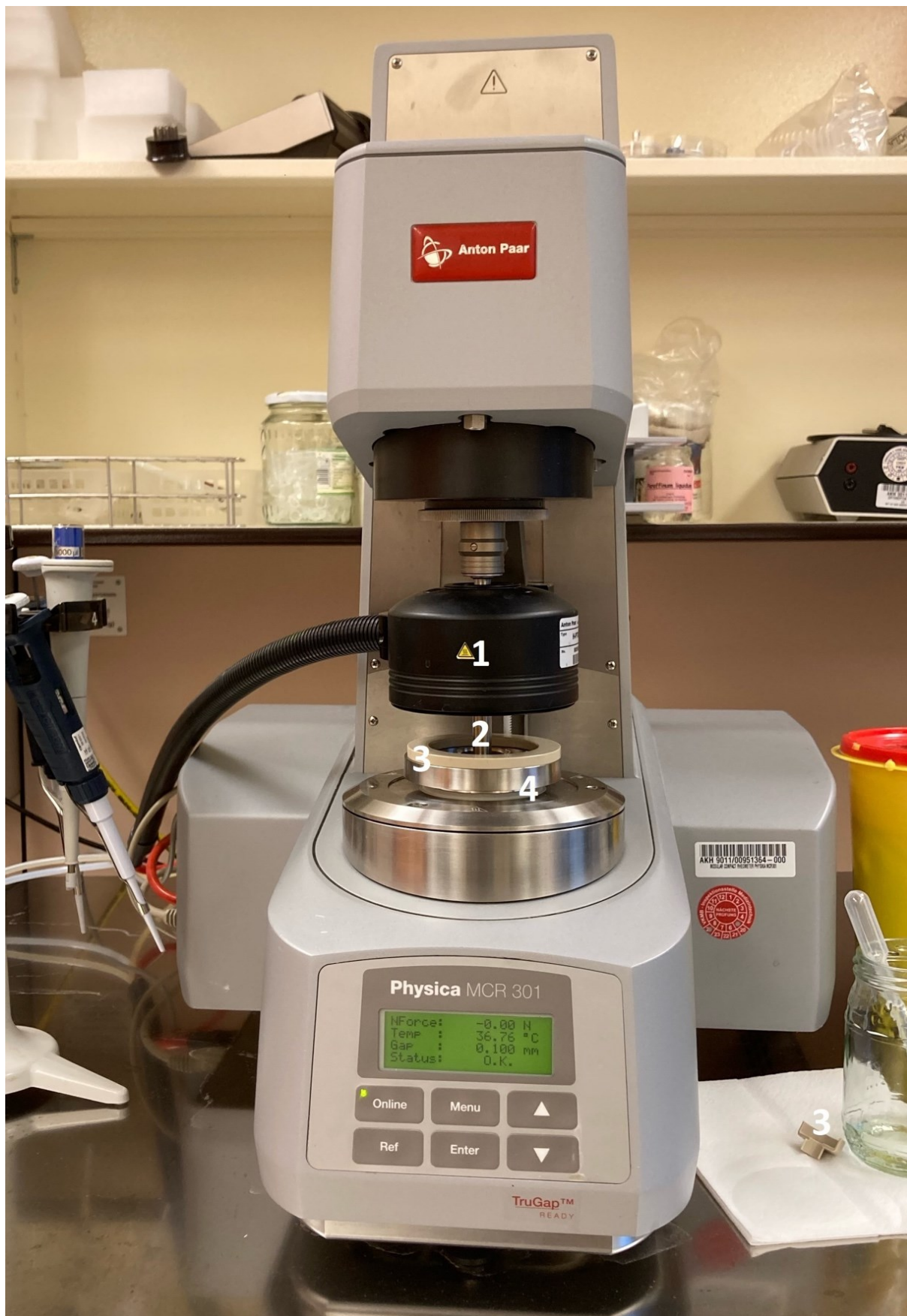
Figure 3.2.: Exemplary setup for the test runs. The most important components are numbered and explained on the following page. Please find more detailed information regarding manufacturing, operative parameters and technical specifications in the product manual “MCR 301 series E” provided by Anton Paar®.
